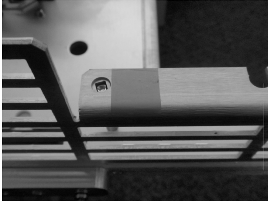
Figure 2 Test Set Deck Chassis with Mylar Tape Installed
